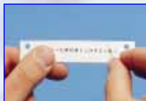
Apply label to cable marker and adhere overlamine
